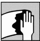
Surface cleaning; remove any surface contamination prior to the application of the solvent borne topcoat using an appropriate surface cleaner.
