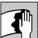
Surface cleaning, remove any surface contamination prior to the application of Priming Filler 680 Grey using appropriate surface cleaner. *Where bodyfiller is exposed, avoid contact with water (e.g. waterborne degreaser).*
